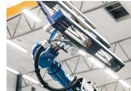
Robots can also be used in other parts of the production, e.g. for sorting pallets according to type.
