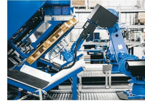
The robot and dismantler system are mounted on a steel platform, which means that it can be easily relocated if the needs of the business change.
