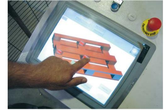
Elements are simply selected for removal from a touch screen at the inspection station before passing into the robot cell.
