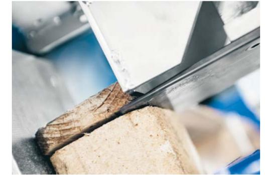
A combination of hydraulic knives cuts and separates the blocks and boards. The waste material falls to a belt conveyor to be disposed of outside the robot cell.
