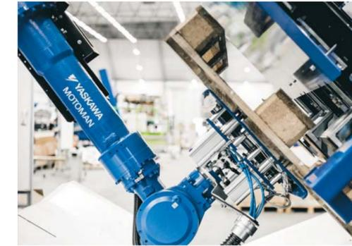
The MOTOMAN robot picks up the pallet and puts it in the dismantler in the correct position for removal of the parts identified in the inspection.
